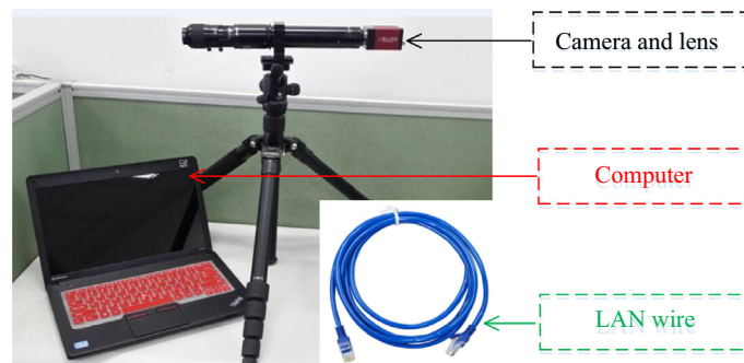
Fig. 2. Vision-based system for multi-point structural displacement measurement.
