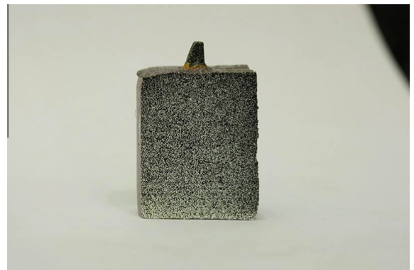
Fig. 2. An implant-PMMA sample prepared for testing in the Tinius Olsen equipment.
