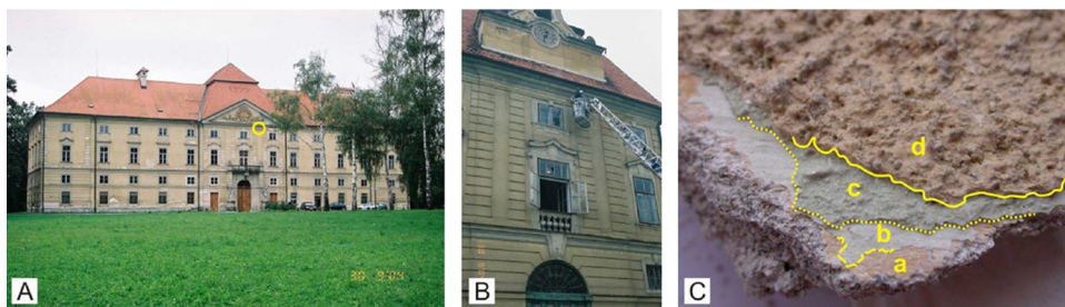
Fig. 1. A view of the north-facing facade wall of the Novo Celje Baroque Mansion, showing (A) one of the sampling locations, (B) the sampling work in progress, and (C) part of the sample from the facade wall.
