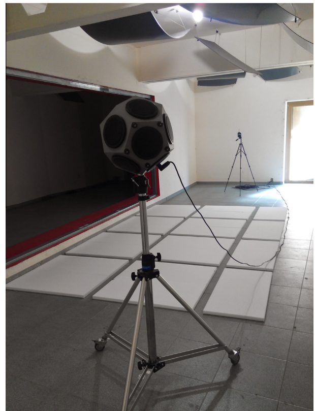
Fig. 2. Test in reverberating room.
