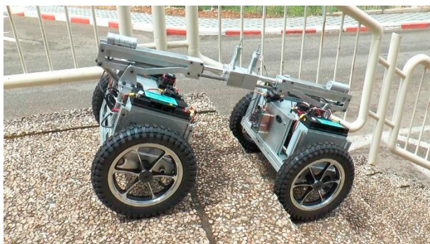
Fig. 1. Two inverted pendulum type robots connected together for stairs climbing
