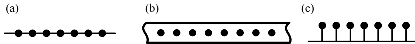
Fig. 1. (a) line type, spheres on wire; (b) line type, cups in belt material (c) comb type, spheres on wire.
