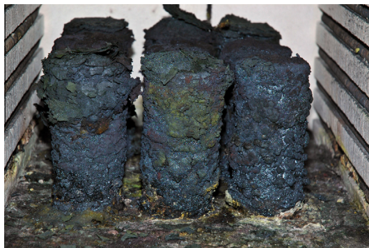
Fig. 1. Photograph of crucibles at the conclusion of the 1000 h static test.
