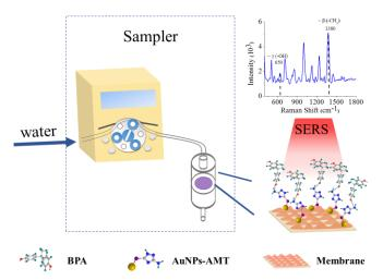
A dual-functional membrane with enrichment and resonance amplification property, combined with an automatic sampler was designed for bisphenol A detection by surface-enhanced Raman scattering.
