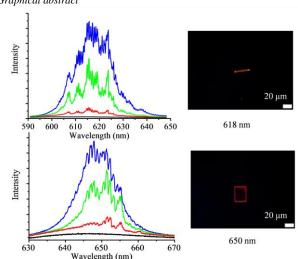
One-dimensional (1D) microwires and 2D microdisks of DMF-HPPO have been selectively prepared by controlling the solution polarity. Tunable amplified spontaneous emissions are achieved and 1D microwire demonstrates sharp splitting photoluminescence peaks around 618 nm, while 2D microdisk shows a red-shifted emission central at 650 nm.
