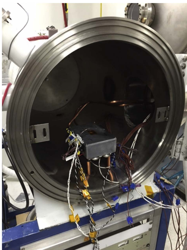
Fig. 2. Vacuum chamber with supercapacitor cells in place (contained in steel chassis box), prior to closure of chamber.
