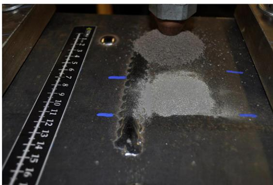
Fig. 1. Addition of alloying elements on CCO's by submerged arc welding.
