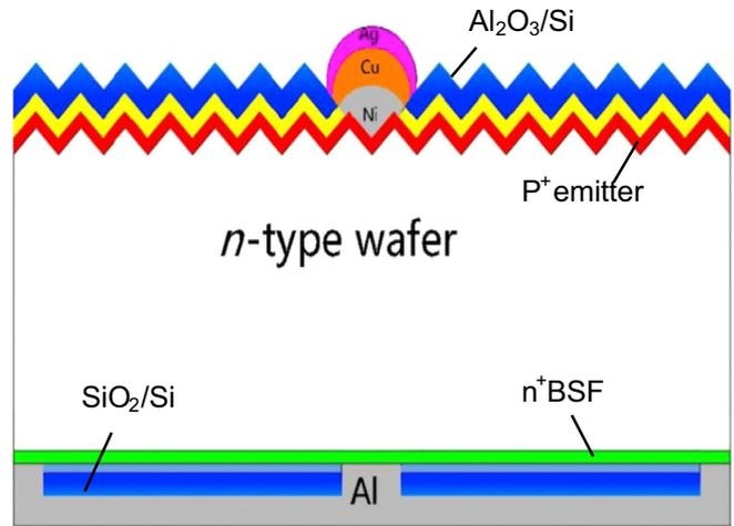
Fig. 1. Schematic cross section of the front junction n-type PERT cell structure.
