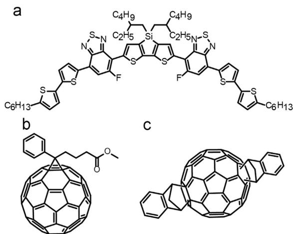
Fig. 1. Molecular structures of (a) DTS(FBTTh<sub>2</sub>)<sub>2</sub>, (b) PCBM, and (c) ICBA.
