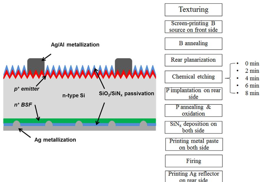
**Fig. 1.** Schematic structure of n-type PERT (passivated emitter, rear totally-diffused) cell and the process flow.
