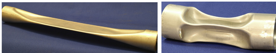
(b) Mode 2 collapse
