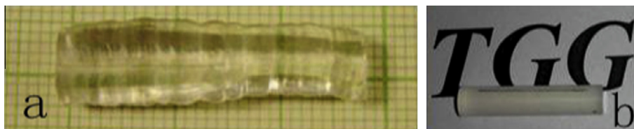
Fig. 2. The as-grown single crystal with the 10 \text{ mm} \times 30 \text{ mm} by the FZ method (a) and (b) the commercial TGG 2 for further measurement in the same apparatus with TGG 1.
