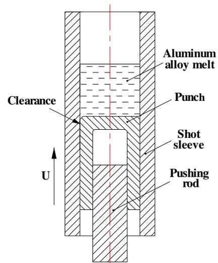
Fig. 1. Injection mechanism.
