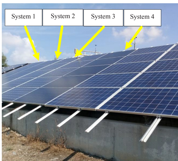
Fig. 1. PV systems installed at the outdoor test facility of the University of Cyprus (Makrides et al., 2013). All modules were mounted in an open rack, same orientation and arrangement within a planar surface. Additional PV modules were installed to fill out the remaining open area of the planar surface in order to allow identical exposure conditions.
