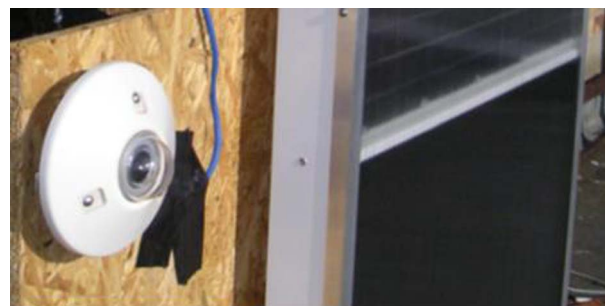
Fig. 2. Total irradiance sensor CM 11 mounted vertically, in line with the mounted solar-air collector.
