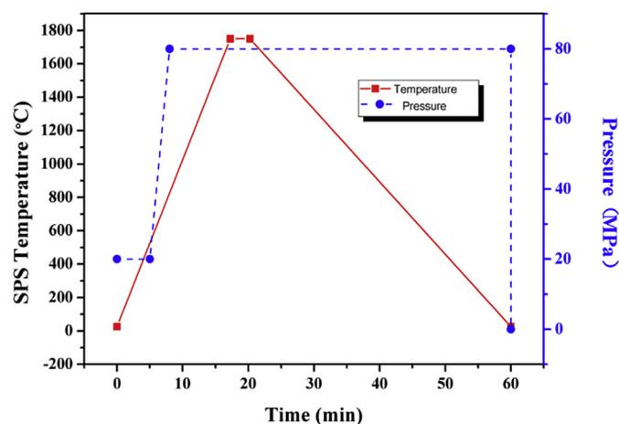
**Fig. 1.** Schematic heating cycles for sintering process.
