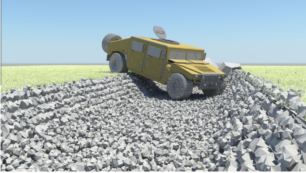
Fig. 1. A HMMWV traversing a deformable terrain modeled using the discrete element method (DEM).
