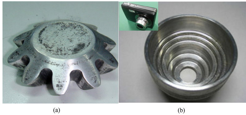
Fig. 1. Photos of magnesium alloy AZ31B applications: (a) spur bevel gear [1], (b) digital camera barrel [2].
