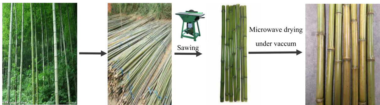
Fig. 1. Schematic illustration for drying round bamboo by VMD method.
