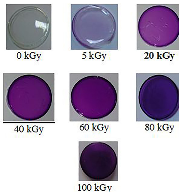
Fig. 1. Color change photos for PVA/Ni 2+ films at different irradiation doses.
