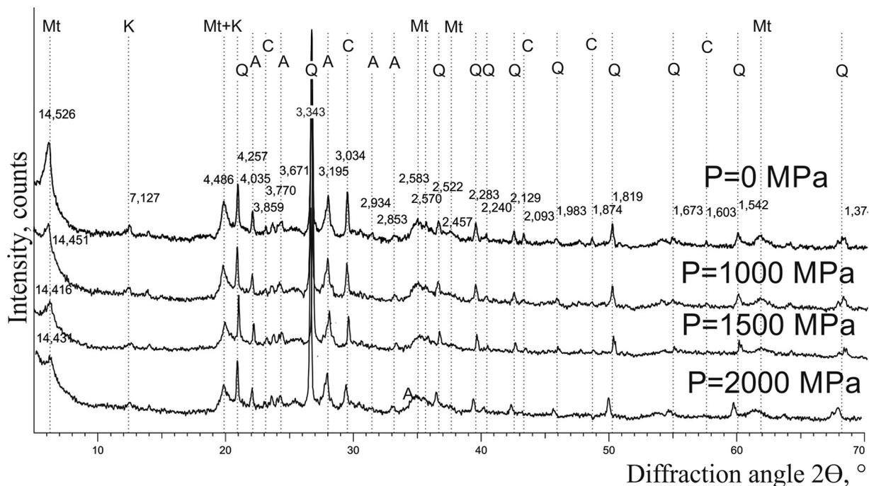
Fig. 1. XRD patterns of bentonite: initial and effected by pressure. Mt. – montmorillonite, K – kaolinite, Q – quartz, A – albite, C – calcite.
