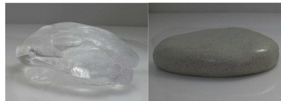
(a) P-silicone gel without abrasive (b) P-silicone gel with abrasive
