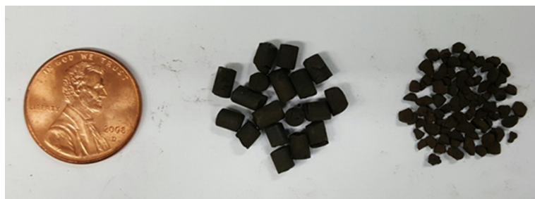
Fig. 1. Fabricated MnO_2/PbO/Al_2O_3 catalysts (center: 1/8 inch catalysts, right: 1.18–2.00 mm catalysts).
