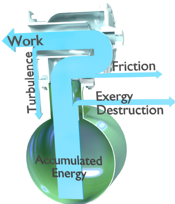
Fig. 2. Distribution of energy losses in a pneumatic pulsator.
