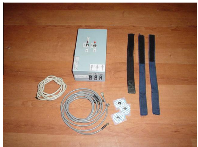
Fig. 4. Cabinet containing the electrocardiograph and the USB communication device and its accessories: USB cable, three-wire bipolar derivations for three surface electrodes and three bands of adjustment.
