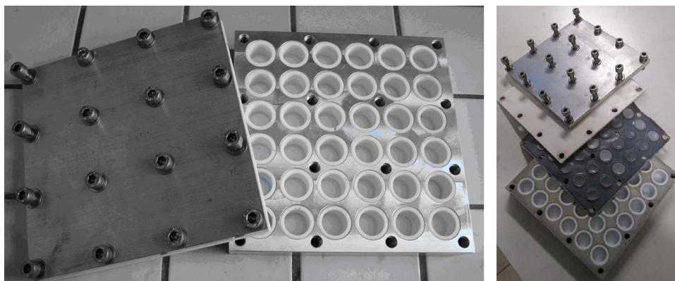
Fig. 1. Image of the high-throughput system that was used for the hydrothermal precipitation reactions.
