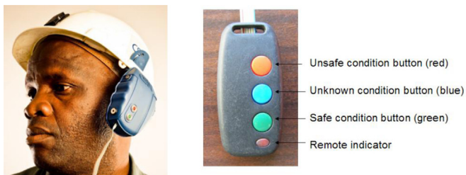
Fig. 1. Photograph showing the attachment of the ESD to a miner's hard hat for operational use (left), and the training dongle (right) that enables the user to label training data recorded. Note that the entire system consists of the headpiece and dongle shown in the figure. (For interpretation of the references to color in this figure, the reader is referred to the web version of this article.)
