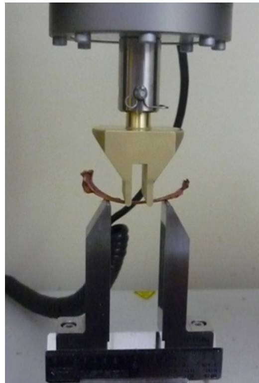
Fig. 2 – A piglet rib fitted into a custom made four-point bending jig.
