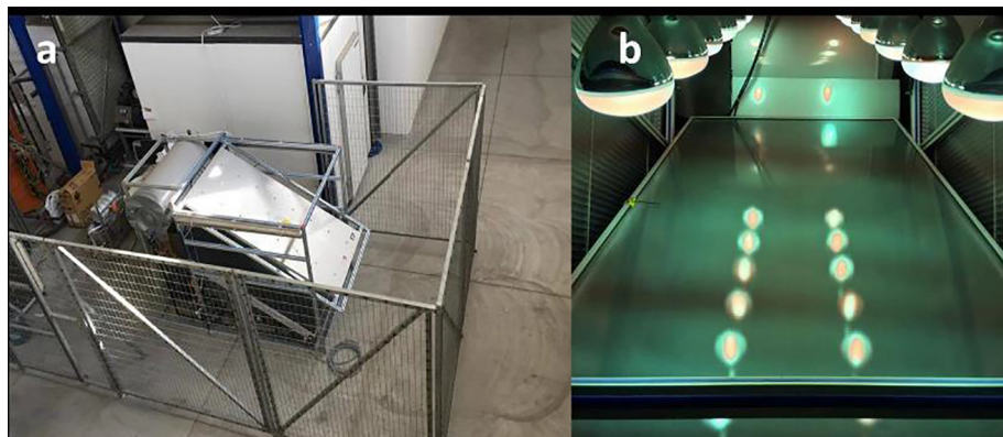
Fig. 1. The examined FPC collector a) The total experimental setup b) View of the lamps.
