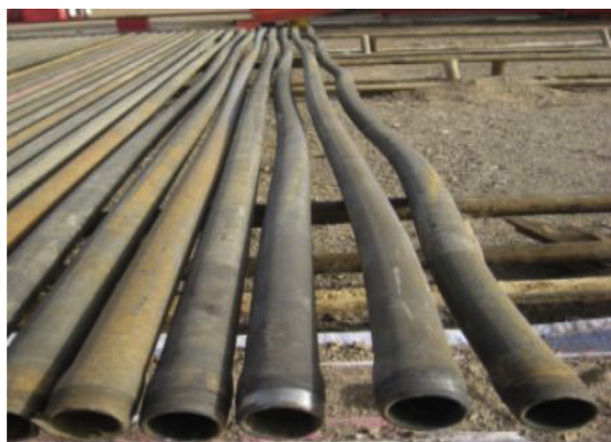
Fig. 2. Deformation of downhole tubing string.
