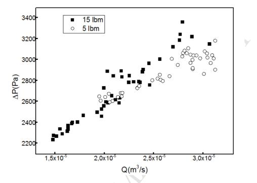
Flow rate as a function of the pressure drop of the suspensions of fine laminar calcium carbonate at 5lbm/bbl and 15 lbm/bbl through a 10 mm fracture.
