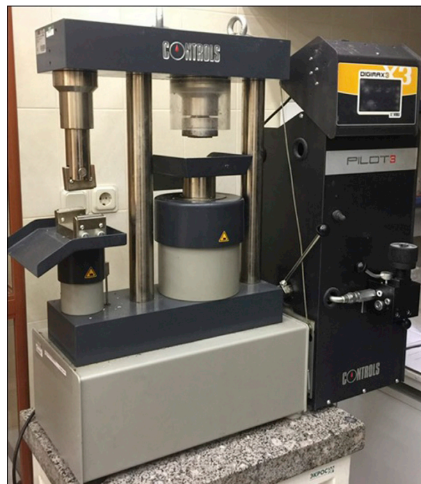
Fig. 3. PILOT compression-flexural cement tester.
