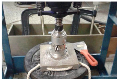
Fig. 1. Cylindrical mold with mechanical compression.
