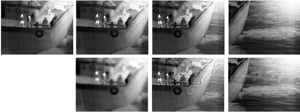
Fig. 1. Examples in the infrared sequence processed by Scribner's algorithm [1]. The top row is the original images and the bottom row is the corresponding corrected images. From the left to the right: the first frame of the infrared sequence; the frame after the scene remains stationary for a while; the frame after the scene motion resumes; the frame after the scene keeps motion for hundreds of frames.
