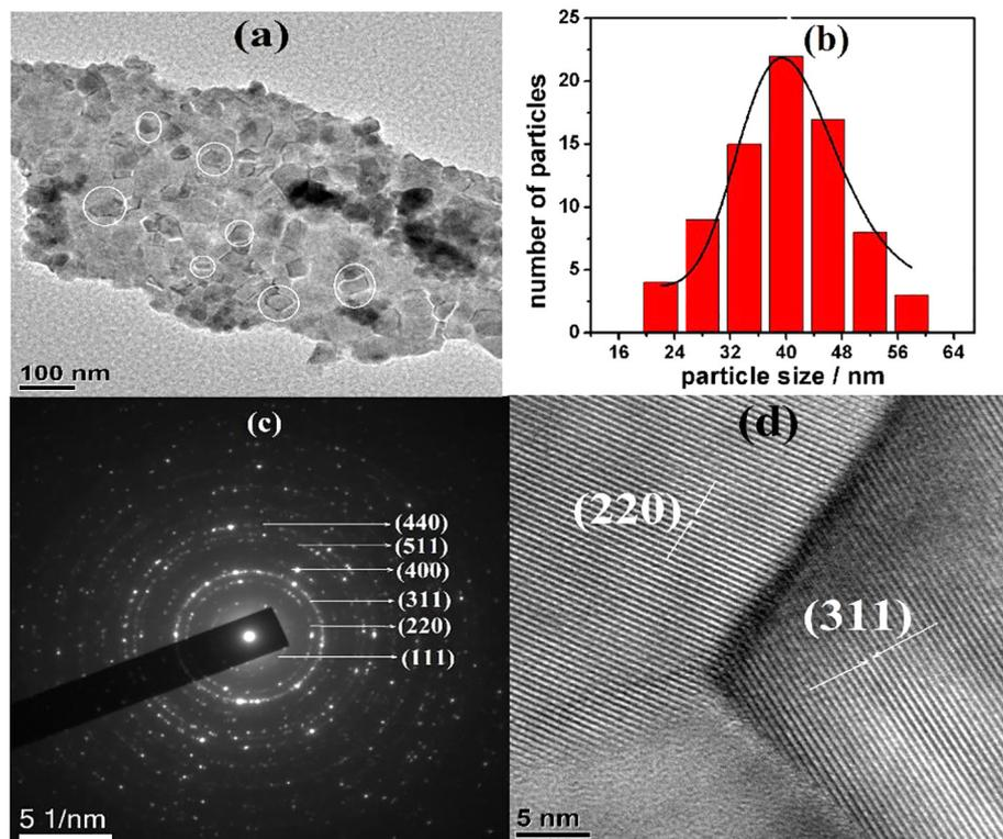
**Fig. 1.** (a) TEM micrograph, (b) particle size distribution with log-normal fitting of the micrograph of Fig. 2(a), (c) selected area diffraction (SAD) pattern, (d) HRTEM lattice fringes of Y15 sample.
