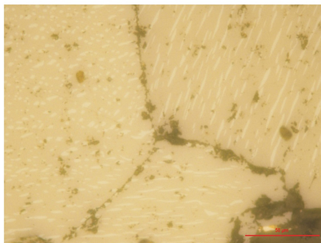
Fig. 1 – Reflected light Microscopic photographs for Abu Ghalaga ilmenite ore showing (a) Minute hematite lamellae segregated within the ilmenite host, and (b) Small grains of hematite are exsolved and segregated at the borders of ilmenite grains.
