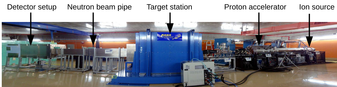
Fig. 1. Entire view of RANS. This is about 15 m in total length, consists of an ion source, a proton accelerator, a target station, a neutron beam pipe and a camera box.
