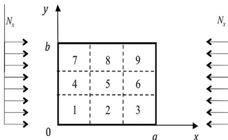
Fig. 1. Plate geometry and load condition. The broken lines and the numbers are explained in Section 5.
