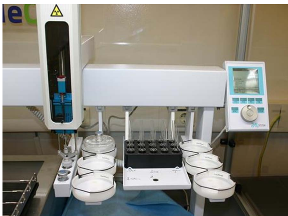
Fig. 1. Ampoules filling station of the automatic dispensing robot, with different items suspended on the horizontal arm (solvent reservoir, waste vial and wash vial, support for the source tray containing 5 mL ampoules).
