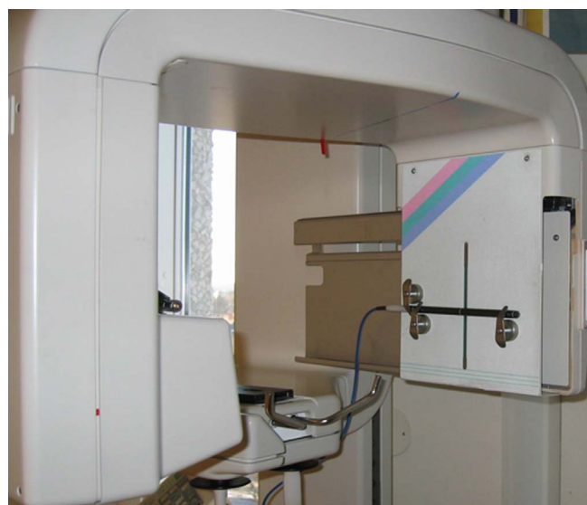
Fig. 1. Setup for the measurement of the kerma area product ( P_{KA} ) using a pencil-type CT ion chamber. Extracted from the IAEA protocol for dosimetry in diagnostic radiology [10].
