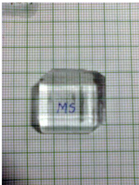
Fig. 1. Photograph of as grown single crystal of AHM from the slow cooling method.
