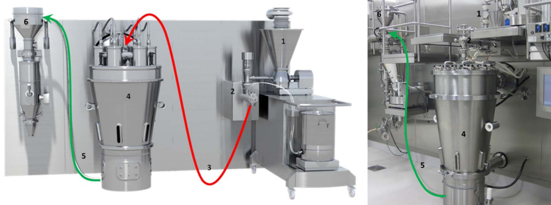
Fig. 1. Horizontal ConsiGma™-25 system (left) and vertical ConsiGma™-25 system (right) with 1. loss-in-weight feeder, 2. twin screw granulator, 3. wet transfer line (only in horizontal set-up), 4. six-segmented fluid bed dryer, 5. dry transfer line and 6. product control unit with option for milling.
