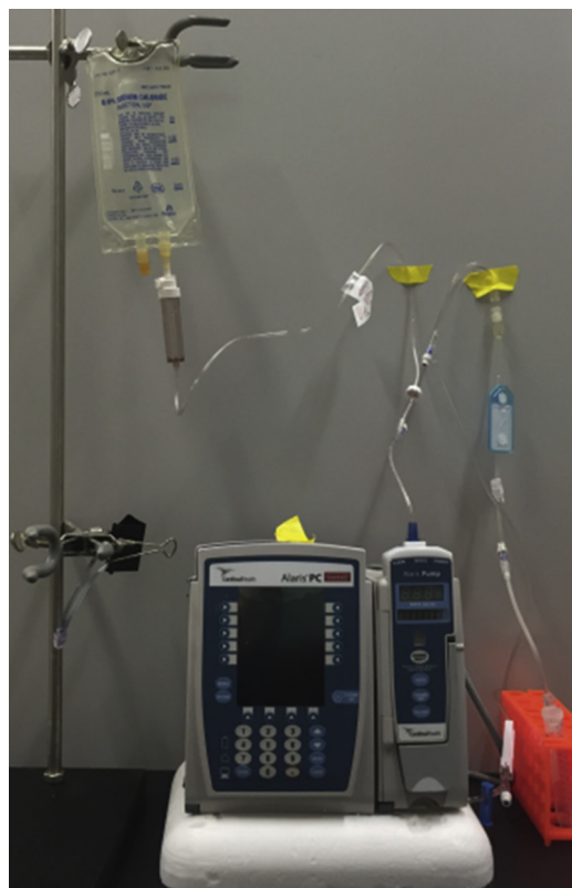
Figure 1. Setup in the laboratory replicating a typical IV infusion system used at the Outpatient Infusion Center of the University of Colorado Hospital.
