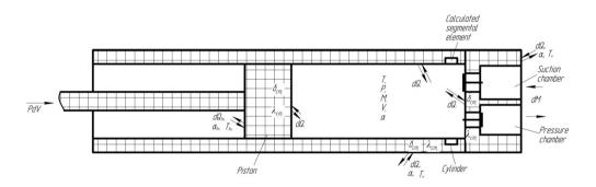
Fig. 1. Design model of the long-stroke low flow stage of the reciprocating compressor.
