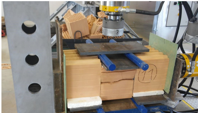
Fig. 1. The test sample for the determination of initial shear strength.
