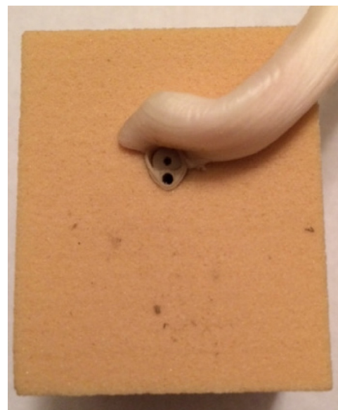
Fig. 2. Placement of the implant within the bone analogue tunnel with the tendon graft. The implant was placed flush to the surface with all suture material completely inserted within the tunnel.
